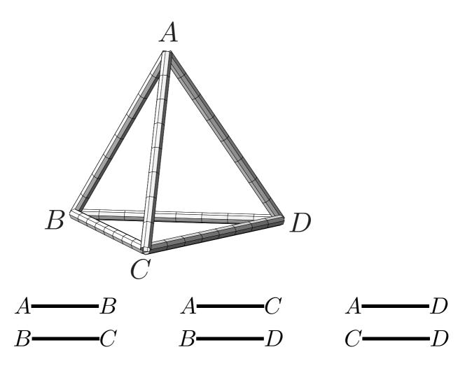
A tetrahedron *is* superrigid: the combinatorial description determines the geometric structure.
